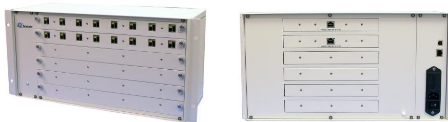
Two Model 600-SM-1-1-32 modules are shown installed in the Model 600-6SL (6-Slot Chassis). Both front (left) and back views are displayed.
